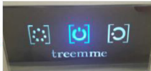
Sistema acceso, LED spenti System on, LEDs off
